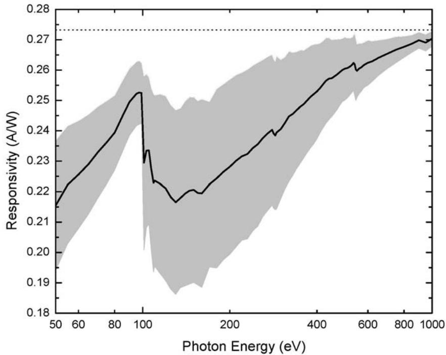
Fig. 5. “Typical” responsivity curve of AXUV-100G diodes in 50-1000 eV photon energy range, compiled from data of 13 diodes. The physical limit of  $S = 1/w$  is indicated as a dotted line.
