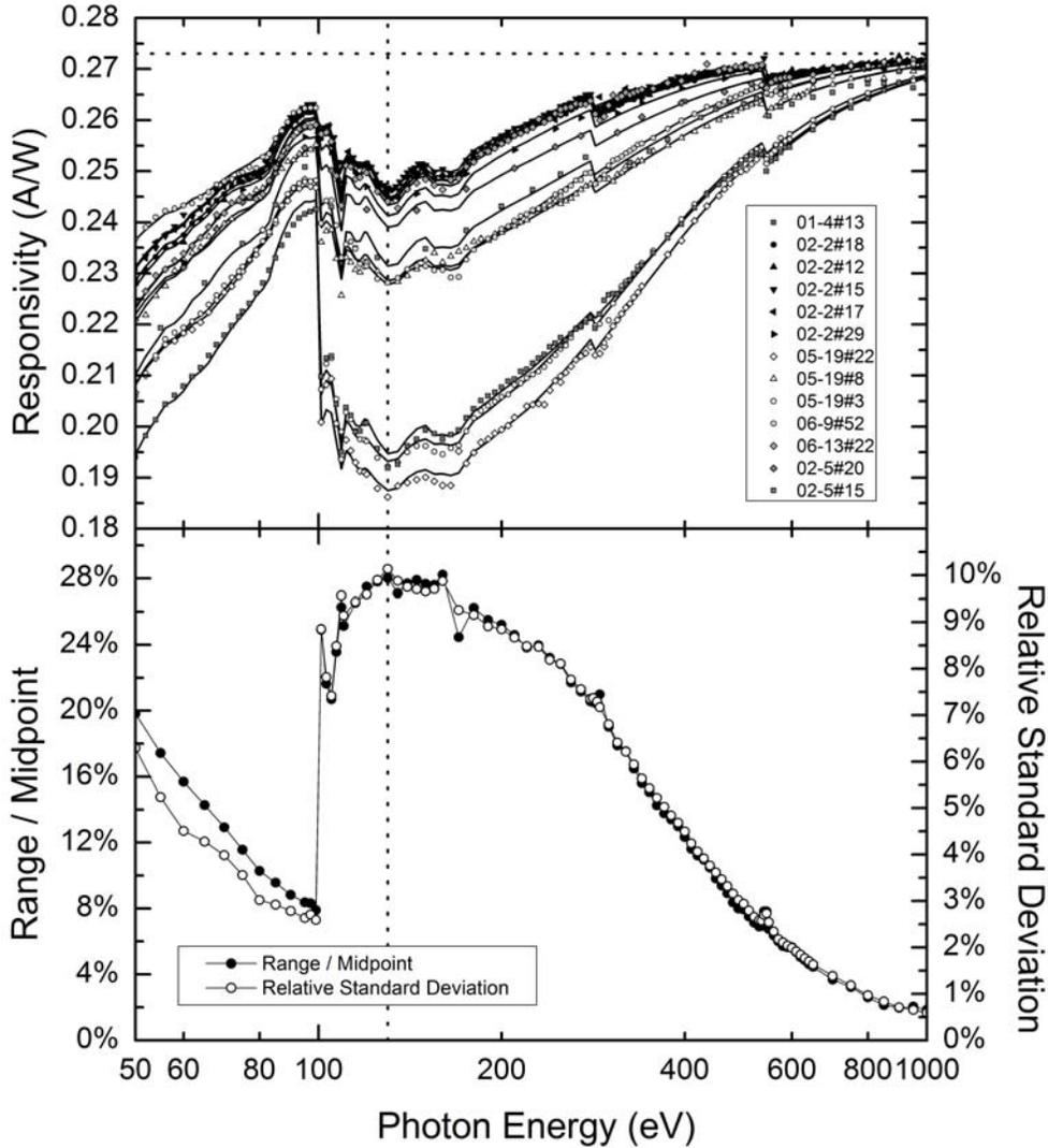
Fig. 3. Measured responsivity curves (50-1000 eV) for AXUV-100G diodes, and variability among the set. The measured responsivity values are shown as symbols, and model functions are drawn through the measured data with fit parameters used as listed in Table 1. The model matches the data to within 3% at each point, whereas the variability among the diodes tested ranges from 1-30% over this photon energy range. Dotted lines are shown at 130 eV and 0.273 A/W for reference.
