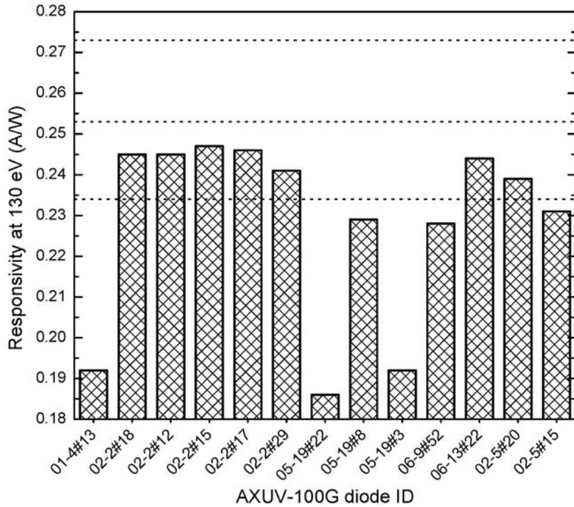
Fig. 4. Responsivity at 130 eV for the diodes under study (each carries 2-5% error associated with it). Reference lines are drawn for maximum possible responsivity, responsivity of dead-layer-free diode, and target performance responsivity as described in the text.
