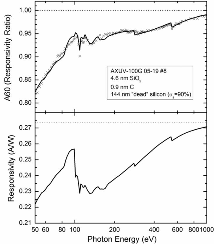
Fig. 2. Example responsivity ratio (self-calibration) data, with corresponding fit, parameters, and responsivity curve for an AXUV-100G photodiode. Reference lines are added for  $A60=1$  and  $S=1/w$  as described in the text.
